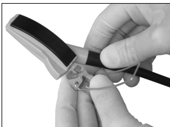
Fig. 8. Mounting needle guide UA1265 (transducer shown without cover).
