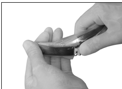
Fig. 9. Smooth and stretch transducer cover when mounting needle guide UA1265
