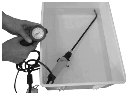
Figure 7. Looking for bubbles in the water tank.
