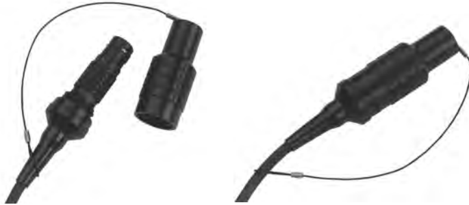
Figure 9. Transducer plug with watertight cover off and on.
