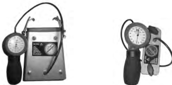
Figure 4. The leakage test kits UA1403 and UA1404.
