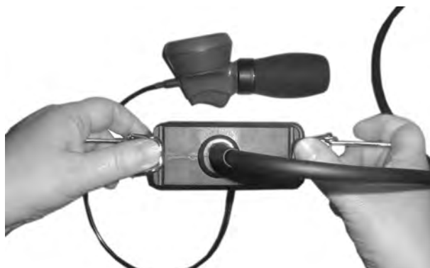
Figure 5. UA1403 – Snapping the locks to attach the box to the plug.
